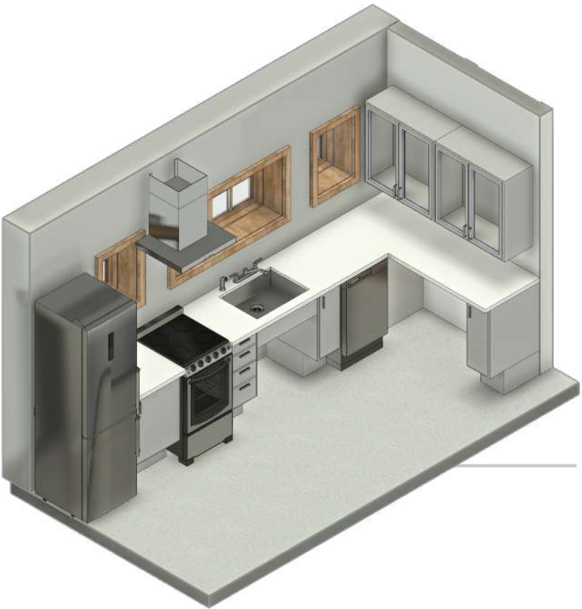
An accessible kitchen, with roll-under sink and roll-under prep areas, as well as casework with large toe-kick clearance to facilitate use by an occupant in a wheelchair.
