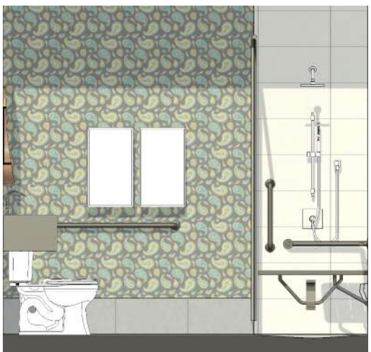
An accessible bathroom including a roll-in shower equipped with fold-down seats, grab bars, and adequate turning radius for wheelchair users.
