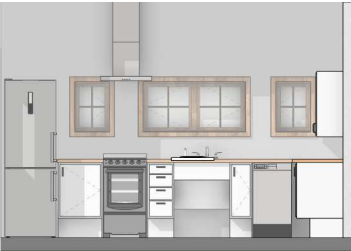
An accessible kitchen, with roll-under sink and roll-under prep areas, as well as casework with large toe-kick clearance to facilitate use by an occupant in a wheelchair.
